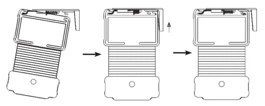
To remove your shade, push the shade towards the window, then rotate the back of the shade down, towards the ground.
